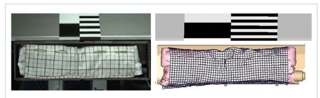
Robustness study of protection cloth; physical test (left); with ESI Virtual Performance Solution (right)
