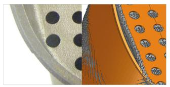
Simulation in ESI Additive Manufacturing shows distortion of the anti-sloshing grid due to incorrect geometry design and build orientation
