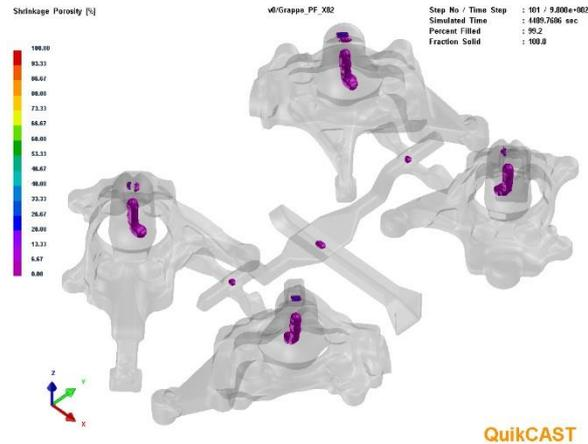
Fig 10: Shows the shrinkage porosity map on 4 of the 8 cavities of the new molding layout (symmetry considered during simulation)
