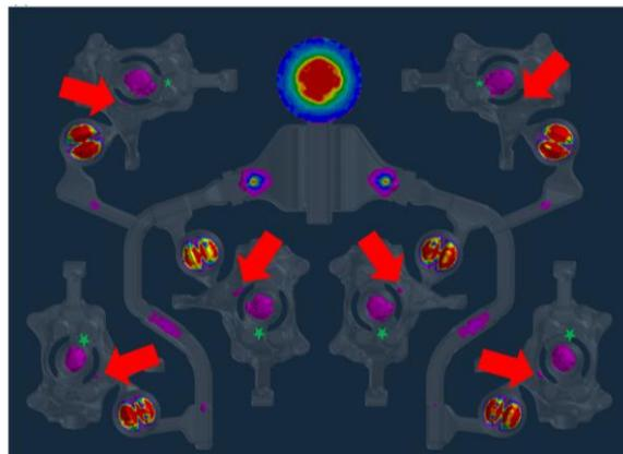
Fig3: Shrinkage Porosity correlation in ESI QuikCAST simulation
