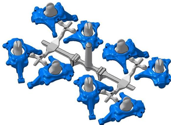
Fig 9: Shows the new 8 cavity molding layout
