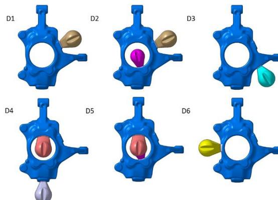
Fig5 : Proposed Feeders for Design Of Experiments
