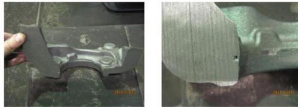
Fig2: Shrinkage Porosity noticed on the cut-sections of the shock absorber arm
