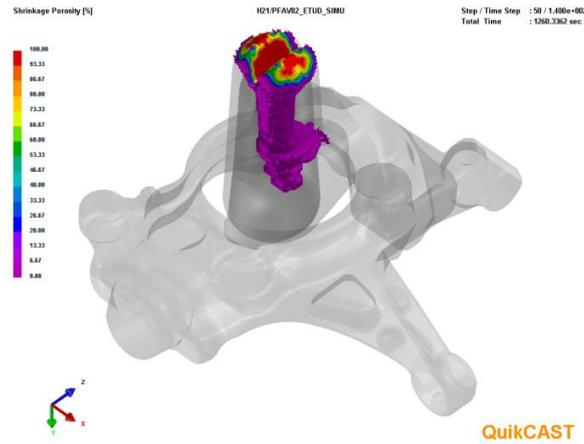
Fig6 : Design 5 shows the best feeder design , with no shrinkage in the casting part
