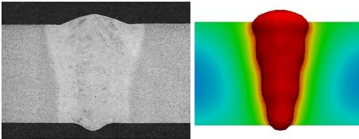
Figure 4: Weld pool cross-section from experiment, and compared to CFD modelling.
