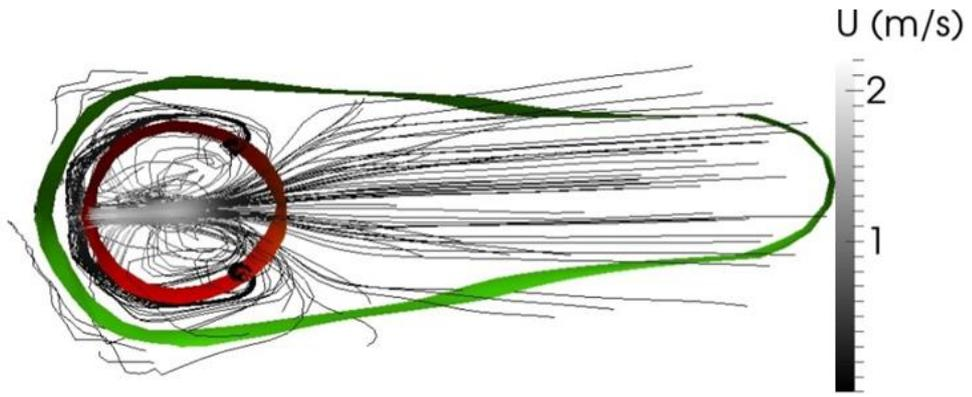
Figure 2: OpenFOAM CFD model showing weld pool (green) and key hole (red) boundaries from top down.
