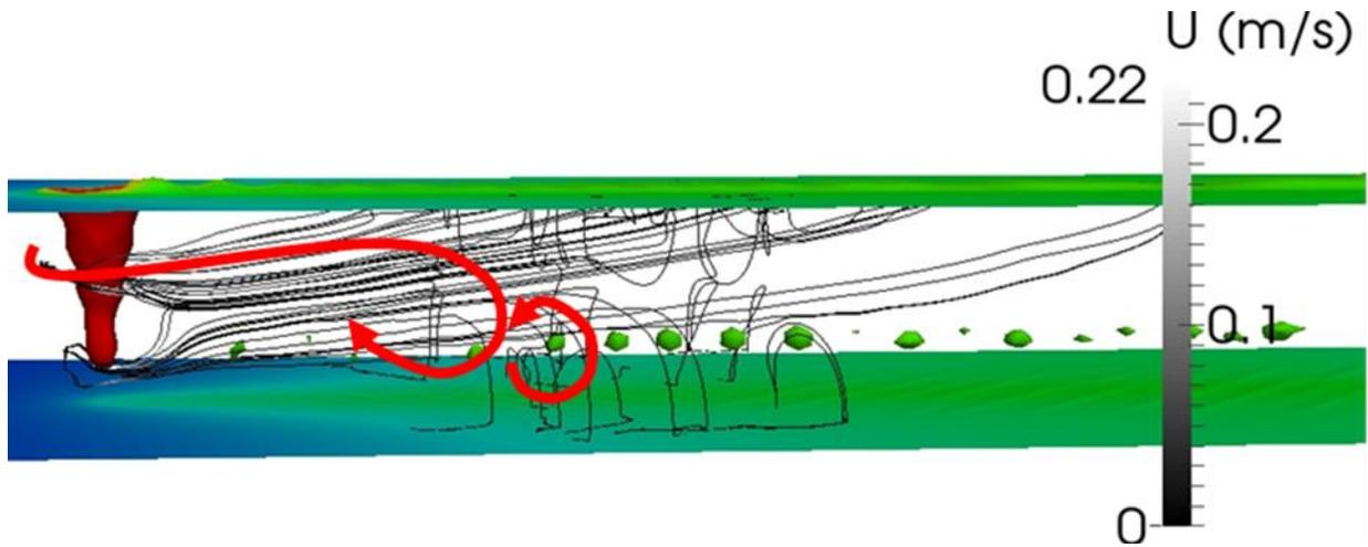
Figure 3: OpenFOAM CFD model showing flow of material within the molten weld pool, and notably the flow around the key hole formation (red), viewed from the side.
