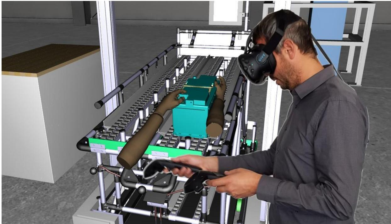
*Image: Assembly process review conducted using ESI IC.IDO 11 with an HTC Vive head-mounted display (HMD)*
