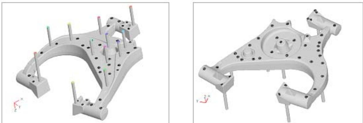
**Figure 8:** Suspension arm core geometry and vents positioning on upper and lower core box.
