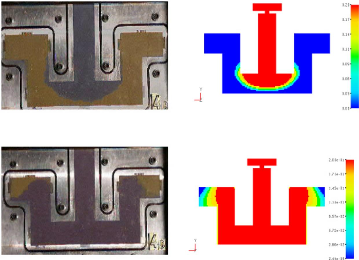
**Figure 4:** Comparison between experiments and simulations for gassing.
