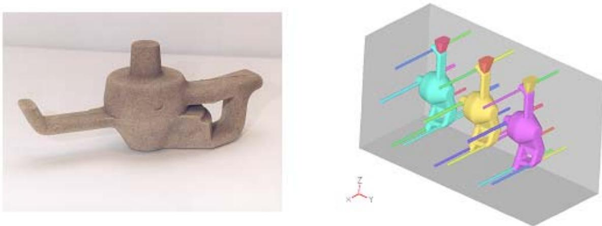
**Figure 5:** Axle core and CAD definition of the core box including core geometries and venting channels (courtesy of Infun).
