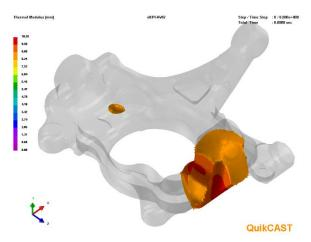
Fig4: Thermal Modulus of the last solidifying regions in the knuckle.
