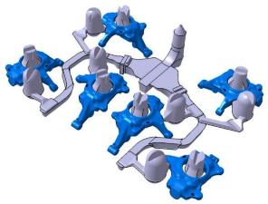
Fig1: 6-cavity mold layout derived from traditional approach
