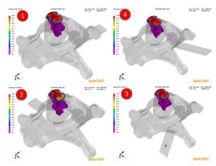
Fig8: Shows identical shrinkage porosity maps with different gate positions
