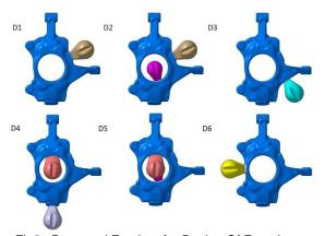
Fig5 : Proposed Feeders for Design Of Experiments
