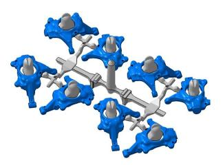
Fig 9: The new 8 cavity molding layout
