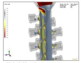
Wall Colmonoy's engineers use ESI ProCAST in conjunction with computer-aided design (CAD) software to streamline the casting process by virtually designing and
