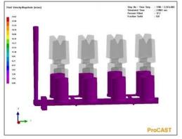
ESI ProCAST fluid velocity model for sand cast roll end bushes in the steel industry. © Image courtesy of Wall Colmonoy Ltd.
