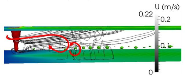
Figure 3: OpenFOAM CFD model showing flow of material within the molten weld pool, and notably the flow around the key hole formation (red), viewed from the side.
