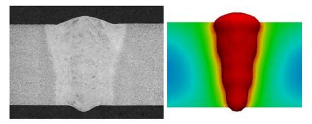
Figure 4: Weld pool cross-section from experiment, and compared to CFD modelling.
