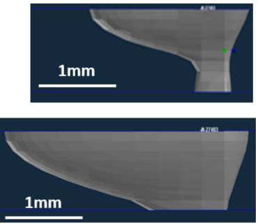
Figure 1: Weld pools produced in ESI SYSWELD using a Cartesian co-ordinate data entry measured from OpenFOAM
