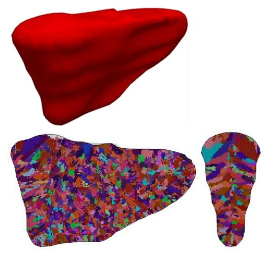
Figure 5: (top) An Extracted weld pool geometry, which can be fed in to the CAFE model in ESI ProCAST (bottom) to predict grain growth and microstructure within the solidified pool – viewed from the side, and from the front.
