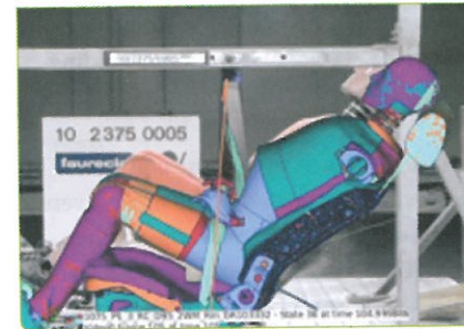
Fig. 5: Rear crash impact for composite backrest: correlation of simulation and experimental test
