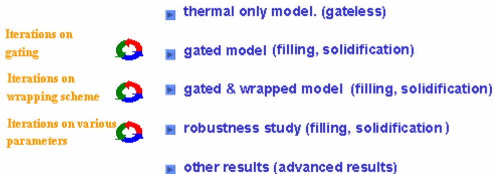
Fig.1 Investment casting modelling methodology
