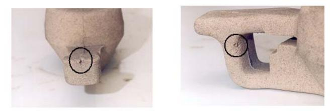
Figure 6: Unfilled areas observed on the axle core (courtesy of Infun).
