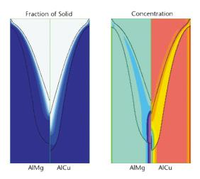
Figure 9: Macrosegregation calculation in a direct chill casting of aluminium. The effect of alloying element on the shape of the melt pool (left), and on the concentration profile (right) is presented. Calculation realised with calcosoft<sup>®</sup>-2D.
