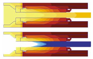
Figure 5: Horizontal continuous casting of copper. The top figure shows the temperature distribution, while the lower figure shows the fraction of solid. Calculation realised with calcosoft<sup>®</sup>-2D.
