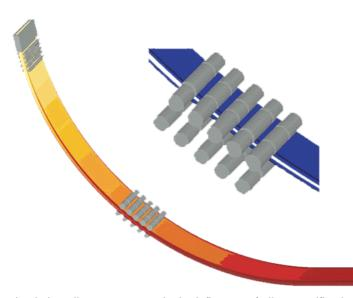
Figure 2: Continuous casting of steel. The larger figure presents the temperature evolution at the surface of the cast metal (yellow is warm and brown is cooler). The magnification shows the evolution of the fraction of solid in a central cross section (blue solid, white liquid). Calculation realised with calcosoft<sup>®</sup>-3D.
