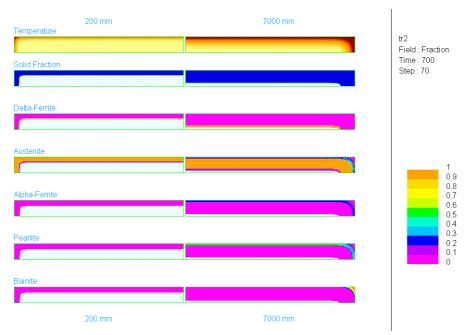
Figure 12: Phase analysis of a steel slab at two different locations during the casting process. Left: analysis at 200 mm
