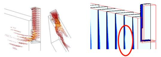
Figure 6: Left: Vectors related to the inlet speed. Bouncing effect against the surface of the mould. Right: Crosscuts showing shell thickness at various locations. Re-melting of the shell highlighted in red. Calculation realised with calcosoft<sup>®</sup>-3D.
