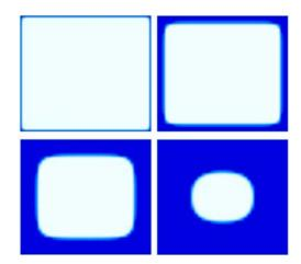
which the metal is gradually changing from liquid to solid, i.e. white to dark blue) can be precisely identified. The influence of the casting speed or of the cooling system design on the positioning of the liquid pool within the graphite insert can be studied.
