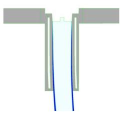
Shell growth can be observed either statically by means of crosscuts in a full 3D calculation or dynamically using travelling sections. Figure 3 represents a lateral crosscut showing the shell thickness at the exit of the mould for a steel bloom. Figure 4 represents several successive transversal crosscuts showing the thickness of the solid layer.
