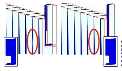
Figure 7: Effect of the nozzle opening size on the surface re-melting. Left: Large nozzle opening, re-melting highlighted. Right: Small nozzle opening, no re-melting can be observed. Calculation realised with calcosoft<sup>®</sup>-3D.
