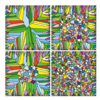
Figure 10: Stochastic modelling of the grain structure in a transverse cross-section of a bloom. The effect on the columnar to equiaxed transition of inoculation, alloy concentration and casting speed is shown. Calculation realised with calcosoft<sup>®</sup>-2D.
