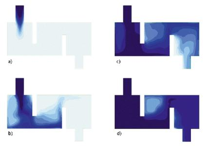
predicted, which eventually corresponds to the section of the final cast product that needs to be removed. This approach can obviously be extended to a tundish supplying several casters, where the time for each caster to have completely reached the new alloy composition might differ. Clearly, the fact that the tundish is emptied in practice to a certain extent before the new alloy is poured, can also be taken into account in the simulation.
