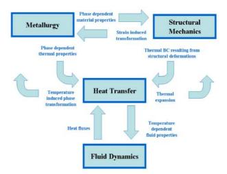
Fig 5. Showing the complexity of the hotforming process interactions.
