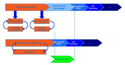
Fig 1. Conventional workflow on top, new proposed workflow based on DIEMAKER for CATIA V5 below – showing clearly the potential time saving.
