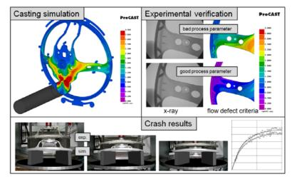
Fig 10: Chaining of casting and crash simulation (Courtesy of Takata Petri)
