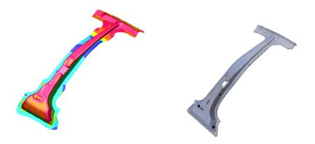
Fig 6. Simulated and real manufactured hotformed B-pillar. Courtesy of AP&T Group.
