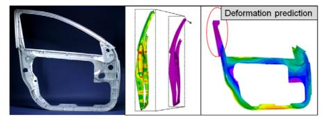
Fig 9: Deformation prediction of a door from Mercedes Benz (Courtesy of +GF+)
