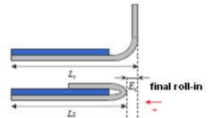
Fig. 4. Final roll-in after the hemming process
