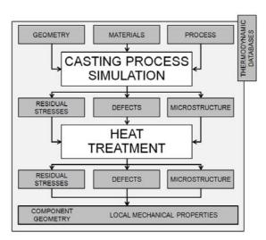
Fig. 8: Casting and heat treatment modelling scheme.
