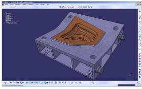
Figure 4: Screenshot of solid tool design after rapid die engineering.
