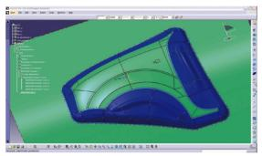
Figure 3: Screenshot of parametric die design with PAM-DIEMAKER for CATIA V5
