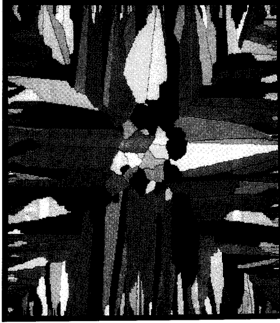
Fig. 10. Final grain structure of an Al-5% Si specimen of uniform temperature, as calculated using the two-dimensional cellular automaton. The parameters for this calculation are the same as those of Fig. 9(b), except for the initial concentration of the alloy.
