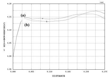
*Figure 5 :* Calculated Mg concentration pofiles at the exit of the real-size DC cast Al-4.06%Mg ingot (Fig. 4) for the cases with shrinkage only (a) and with buoyancy plus shrinkage (b).
