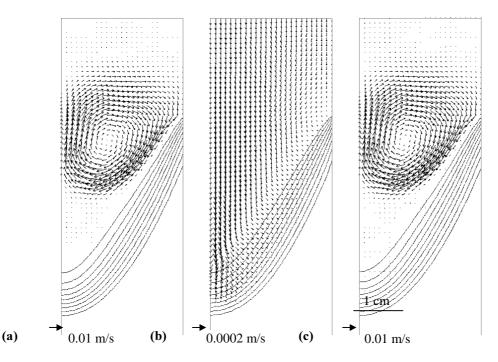
**Figure 2**: Calculated stationary field of the relative fluid flow velocity for a small DC cast Al-4.5%Mg ingot (casting speed :  $1 \text{ mms}^{-1}$ ) with isolines of fraction of solid. a) buoyancy only ; b) shrinkage only ; c) buoyancy and shrinkage. Microsegregation model of Ref. [5] with a Scheil approximation.
