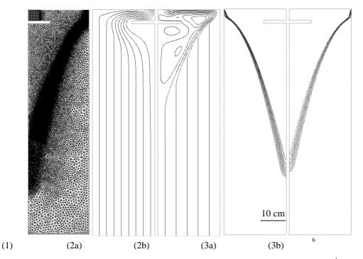
**Figure 4**: Real size DC casting simulation for an Al-4.06%Mg alloy solidified at  $1 \text{ mms}^{-1}$ : Mesh size (1), velocity streamlines (2) and isolines of fraction of solid (3) for the cases with shrinkage only (a) and with buoyancy plus shrinkage (b). Microsegregation module of [5] used with the lever rule. 16417 nodes, about 24h CPU on SG12000.
