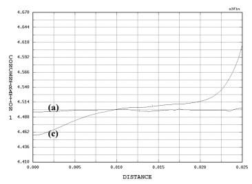
*Figure 3 :* Mg concentration profiles at the exit of the small DC cast ingot for the cases involving buoyancy only (a) and buoyancy plus shrinkage (c) of Fig. 2.
