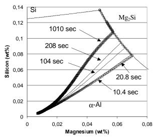
**Figure 3:** solidification paths for five solidification times for an AA6063 alloy.
