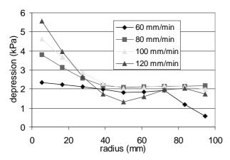
**Figure 10:** steady state depression as a function of the radius for billets 200 mm in diameter cast at various casting speeds.
