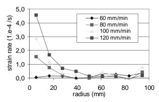
**Figure 11:** strain rate perpendicular to the thermal gradient at the coalescence temperature as a function of the radius for various casting speeds.
