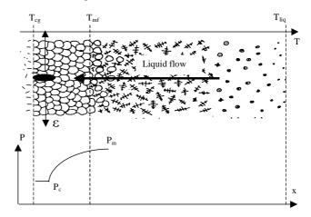
**Figure 2:** schematic of the formation of a hot tear between equiaxed grains as a result of a localized strain transmitted by the coherent dendrites below. The pressure drop in the interdendritic liquid is also indicated.
