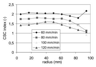
**Figure 12:** CSC index as a function of billet radius in the steady state regime of casting for various casting speeds.
