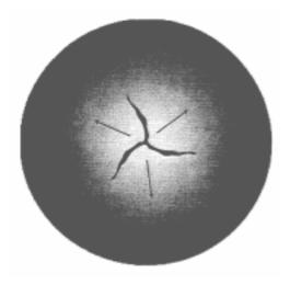
**Figure 1:** central hot tears observed in DC cast aluminum billets [11].
