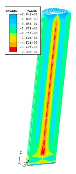
**Figure 8:** computed depression in kPa for a billet 200 mm in diameter cast at 120 mm/min.
