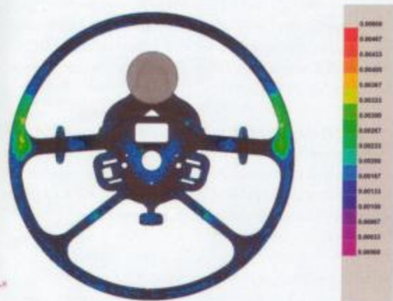
Figure 2 – Shrink porosity indication in the wheel.
