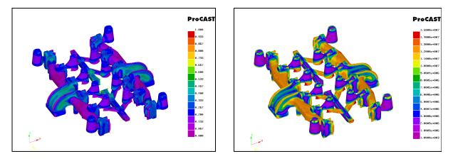
Figure 2: Fraction of ferrite (left), and nodule count (right), provide insight into the mechanical state of the as-cast part.
