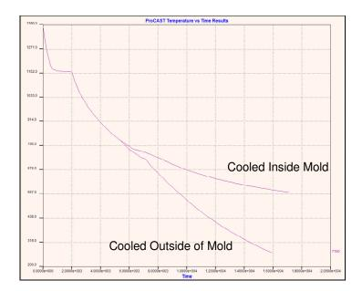
Figure 3: Cooling curves at the same location indicate the cooling rate differences when the part is cooled inside the mold versus when the part is shaken out while still above the solid state temperature.
