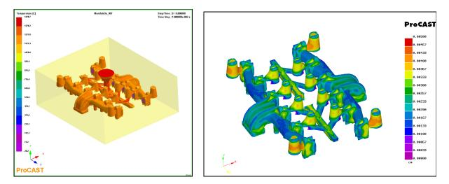
Figure 1: The chemical composition can be varied to identify the optimum mechanical properties configuration (SDAS results of ProCAST<sup>TM</sup> on the right and geometry with the gating, risering and sand mould on the left).
