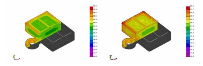
Figure 4: Tensile Strength plots display material property differences between a part that is shaken out after (left) versus before (right) solid state temperature is reached (ProCAST) (Pictures courtesy of Caterpillar, Inc., USA).
