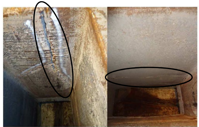
Figure 2: Typical crack pattern on mold after a limited number of ingot production cycles
