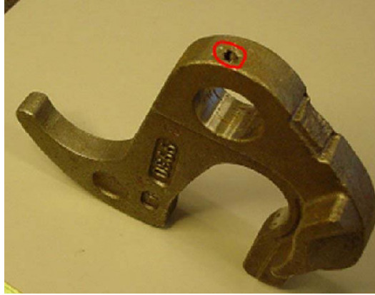
Figure 3. Air/Gas entrapment locations.
