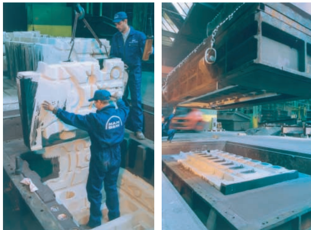
13 cores are putting in the mould
