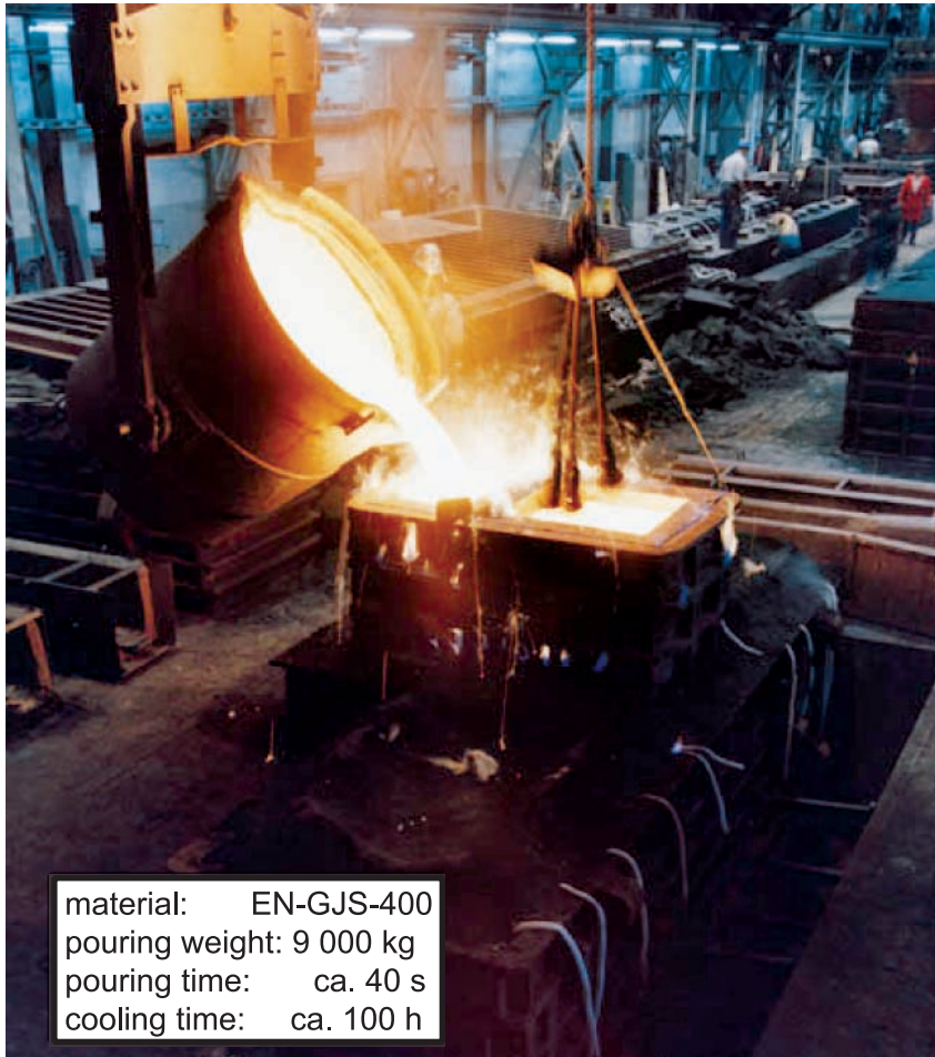
12 Casting the mould.
