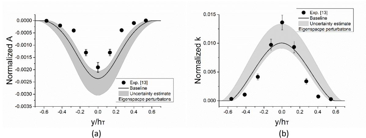
Fig. 3: Uncertainty estimates of eigenspace perturbations on turbulent mass flux velocity (a) and turbulence kinetic energy (b), comparing with the experimental results of [13].
