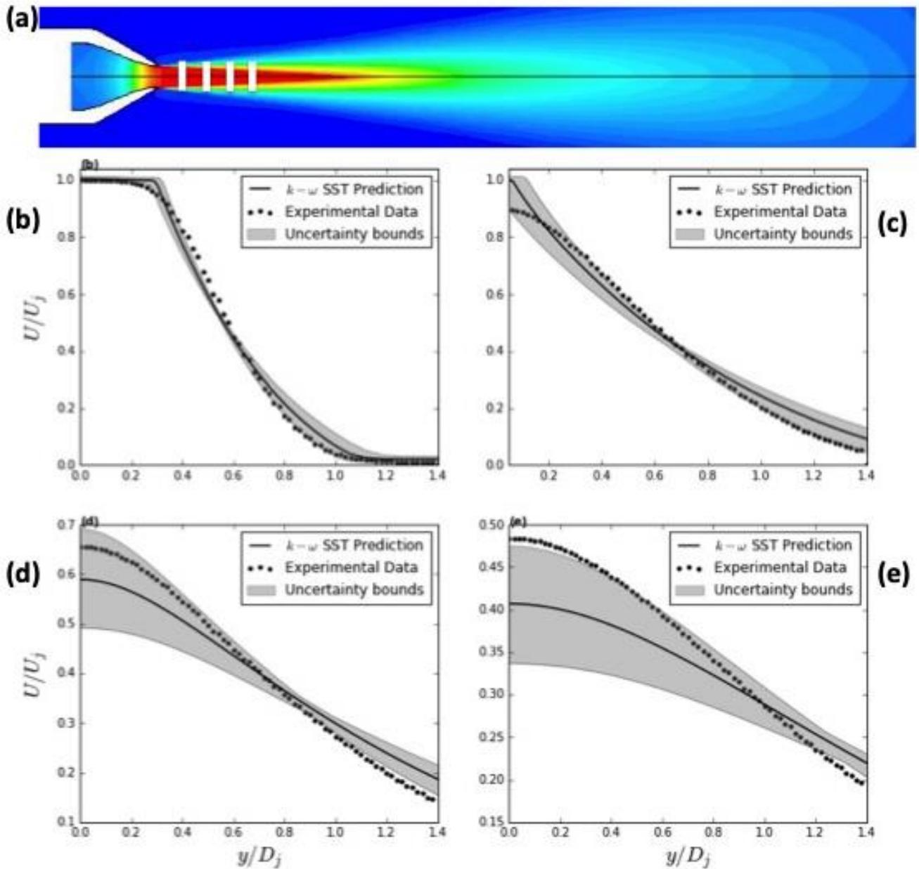
Figure2: Outlining the uncertainty estimates for the NASA ARN Jet. a) Mach number contours, outlining the locations of the mean velocity profiles with white dashes; b),c),d) and e) Outline the mean axial velocity profiles for the NASA ARN heated Jet at  $Ma=0.37$ , delineated at  $x/D=4,8,12$ , and  $16$  respectively.
