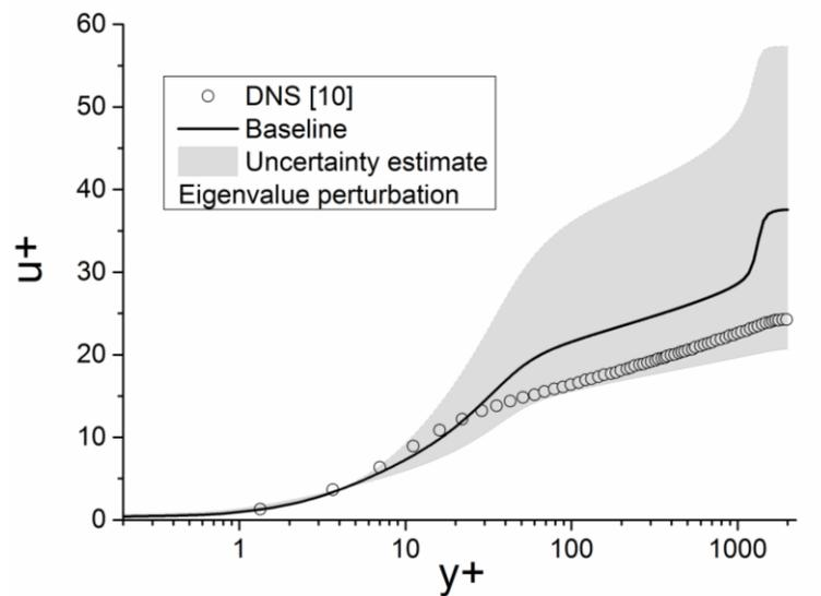
Fig. 1: Uncertainty estimates of the eigenvalue perturbations on mean velocity  $u^+$  for k-epsilon model, comparing with DNS data of [10].
