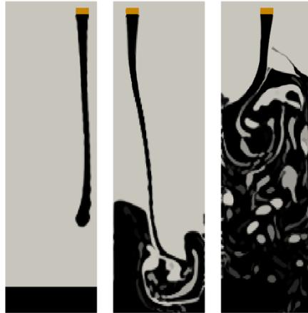
Figure 1 . Results of a multiphase application using the GIB method. Black and grey colours represent regions with two different (Black - high viscous fluid, grey - air). Yellow area represents a moving inlet boundary, which injects high viscous fluid in the domain and is modelled using the GIB method.
