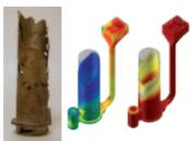
Trial run of partially filled prototype casting vs. Simulation results showing favorable correlation. (Using a different set of parameters than Fig. 2)
