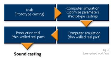
Another part of the project was to develop thin-walled Aluminum industrial parts (2mm). The same principle was successfully adopted.
