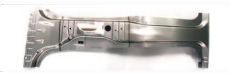
B-pillar stamped from tailored blank with 3 thicknesses and 2 weld lines (visible)
