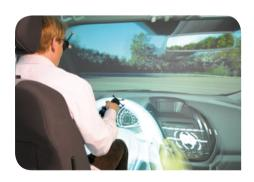
Stereoscopic multiple walls immersive visualization system used in the ergonomic assessment of a car cockpit.
