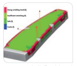
Undesirable effects calculation with straightforward visual output
