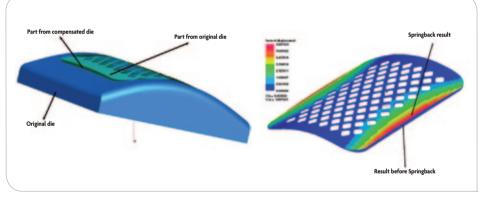
Springback compensation result on die shape (left) and final part (right)
