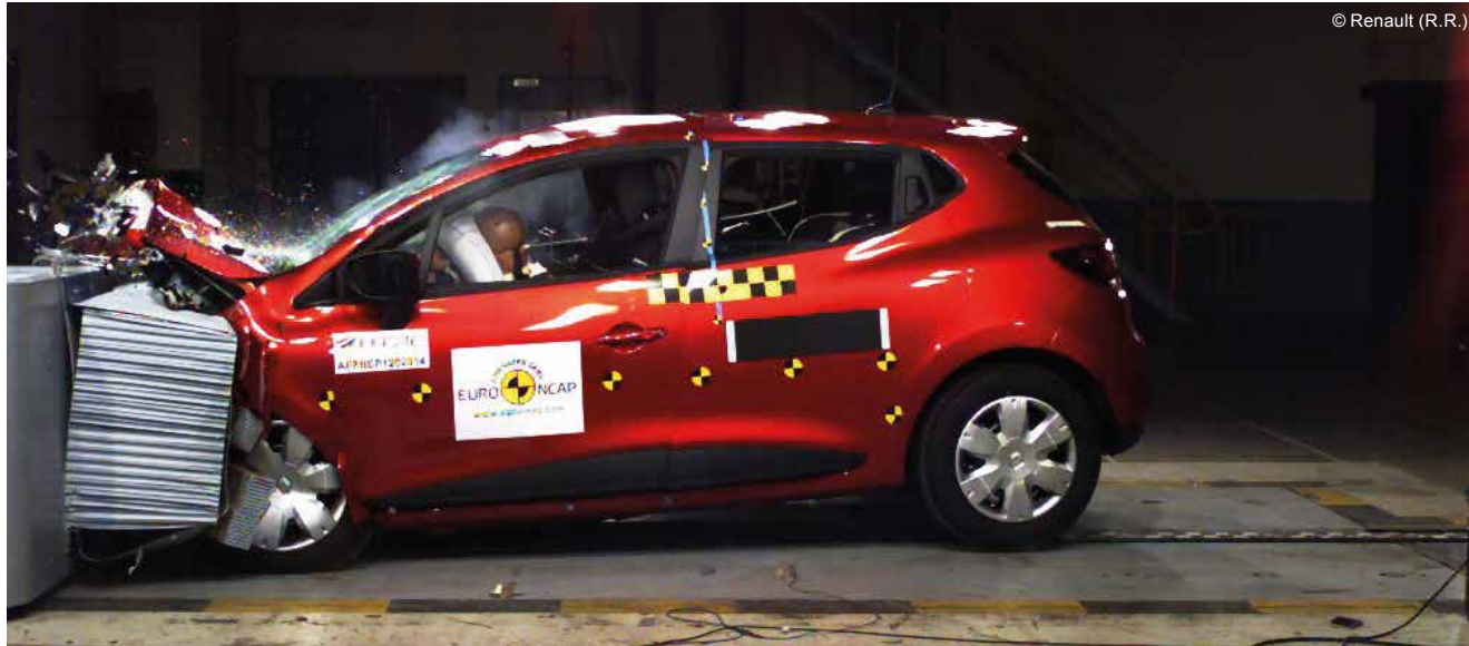
Road safety is one of the cornerstones of Renault's corporate culture and draws on fifty years of research and development. Crash test in 2012 on New Renault Clio.
