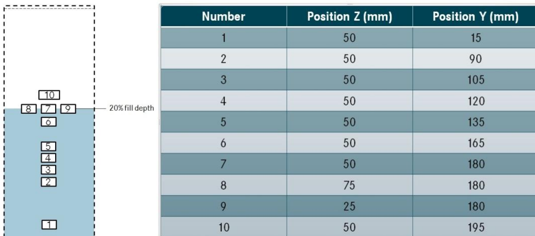
Figure 4: Pressure probe locations
