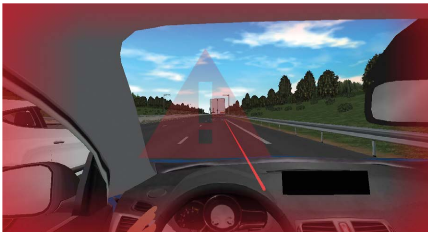
The cognitive model uses the simulated sensors' input to detect changes in the environment (slow truck ahead, passing car,...) and update situational awareness 1 .
