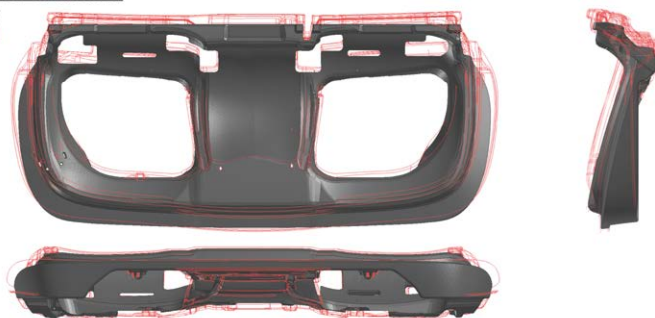
Thermal Shrink Simulation – Distorted Shape
