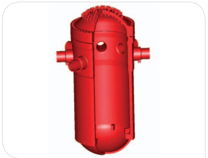
3D SYSTUS/SYSWELD simulation of a reactor vessel Courtesy: AREVA
