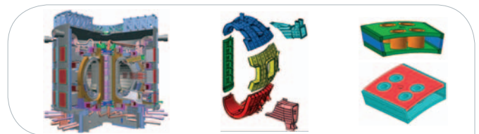
Distortion analysis of the 'Vessel Advanced Technology Segment' (VATS) during electron beam welding assembly
