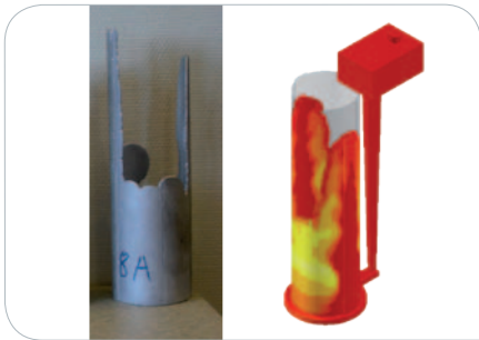
Fig. 2 - Trial run of partially filled prototype casting vs. Simulation results shows favorable correlation.
