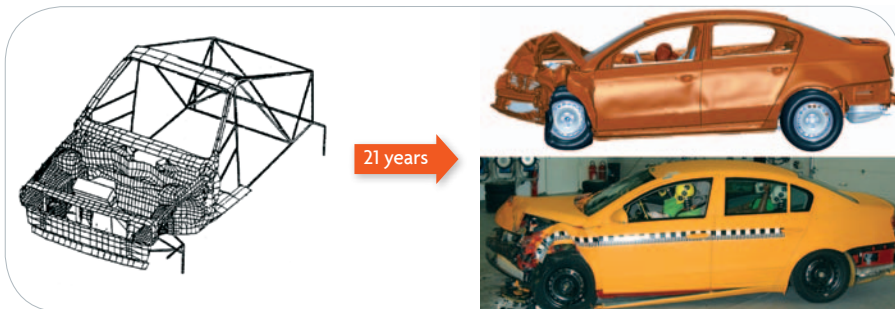
The first full car crash simulation model: The VW Polo – 1985 (left) Frontal impact car model simulation (EuroNCAP certification) - 2006: Courtesy of Volkswagen AG (right)
