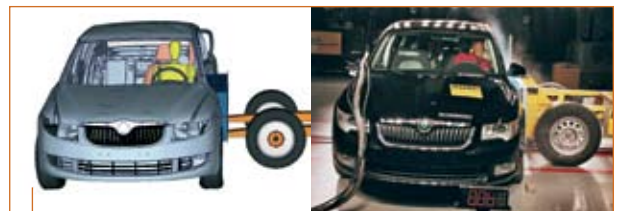
Škoda Superb, side impact with mobile barrier, 50km/h EuroNCAP
