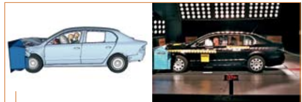
Škoda Superb, frontal impact with deformable barrier, 0°, 40% offset, 64 km/h EuroNCAP
