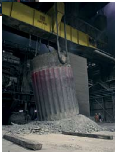
The 300 tons ingot after being taken out of the mold
