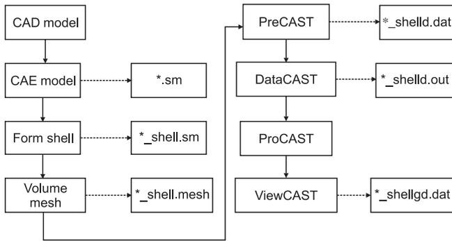
Fig.3: Flow chart of the simulation process based on ProCAST
