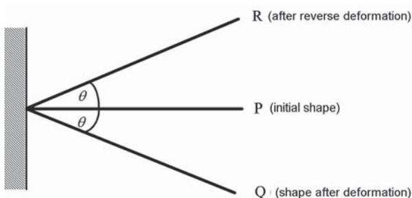
Fig.1: Sketch for the basic principles of reverse deformation
