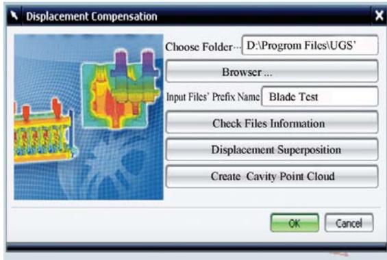
Fig. 9: Interface of anti-deformation system for investment casting
