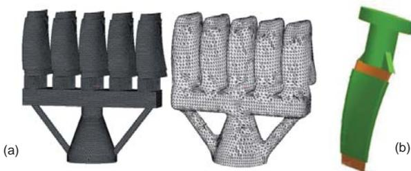
Fig.7: (a) Gating system design and mesh generation (b) The simplification of the typical turbine blade
