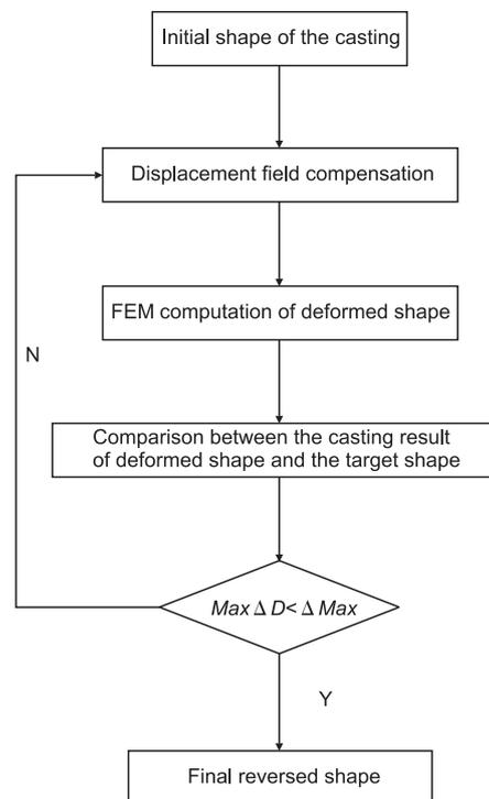
Fig.2: Flow chart of the solution algorithm of the reverse deformation
