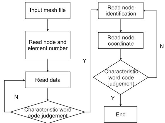
Fig.4: Flow chart of the mesh information acquisition
