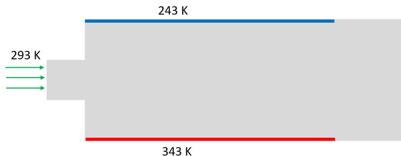
Figure 2. Schematic representation of the temperature boundary conditions.
