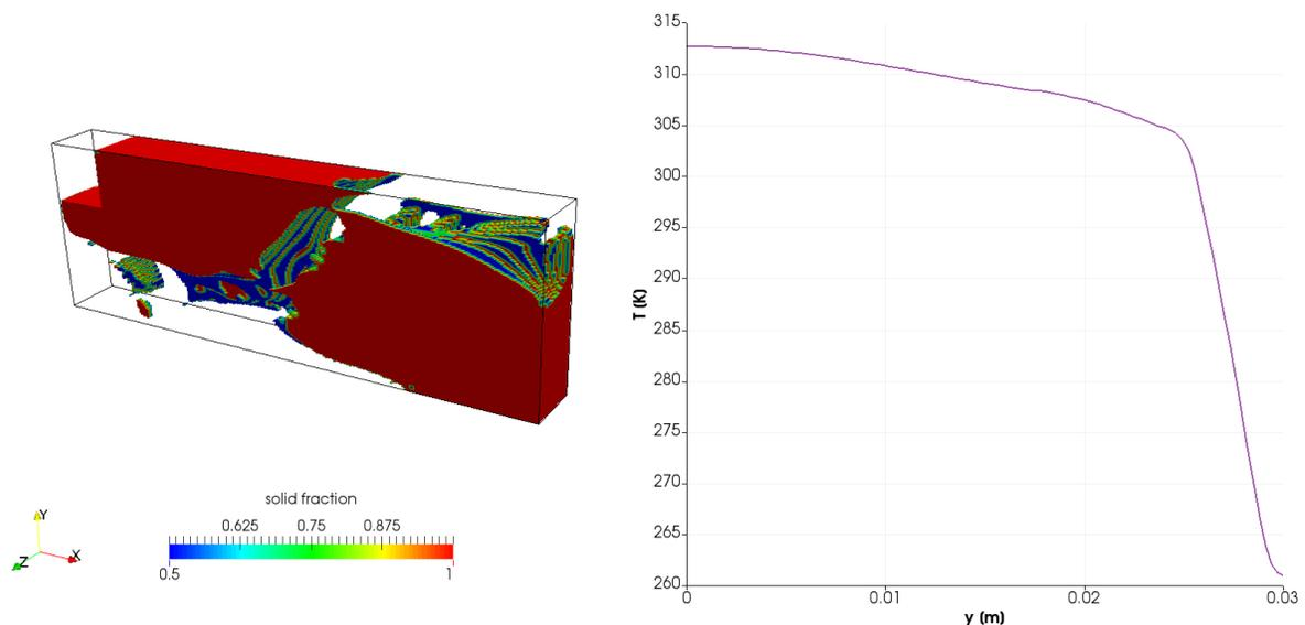
Figure 5. Solid fraction distribution in the 3D domain and T profile along the centerline of the outlet section.
