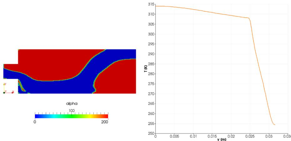
Figure 4. Inverse permeability distribution after the optimization process and T profile along the outlet section.
