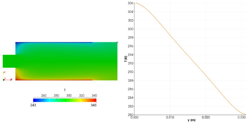
Figure 3. Temperature distribution of the test case and temperature profile along the outlet section.
