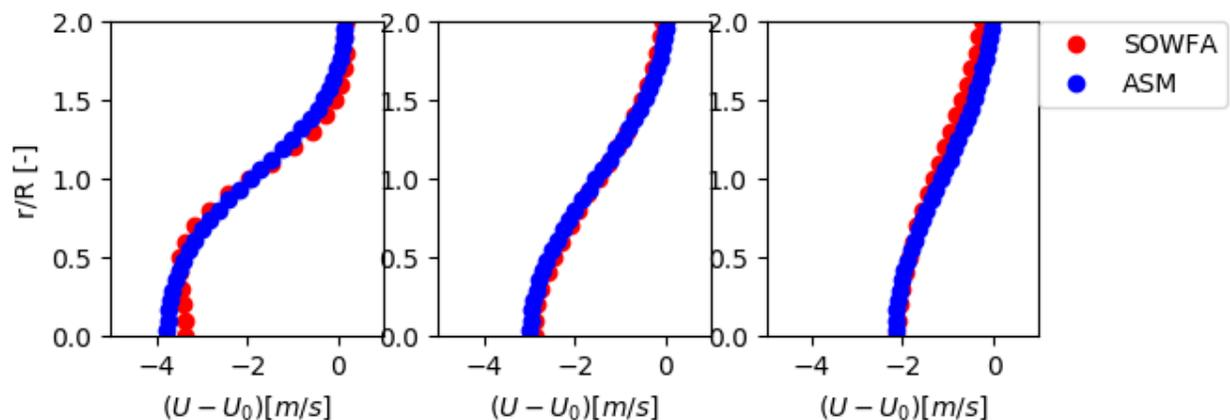
Figure 2: Radial profiles of axial velocity deficits at 2D, 4D and 6D downstream of the wind turbine for the wind velocity of 8m/s and turbulence intensity of 6%
