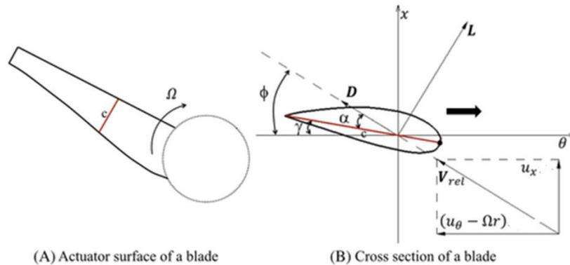
Figure 1: Schematic representation of a turbine blade cross-sectional view of the blade airfoil (image based on Yang and Sotiropoulos [2])
