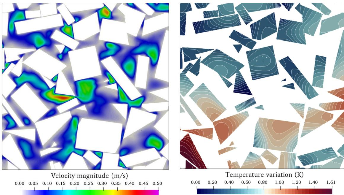
Figure 1 : Velocity (left) and temperature variation (right,  $T(z) - \min(T(z))$ ) at  $z = 27 D_p$ ,  $Re = 10$  across a wood chip bed under constant heat source of  $5.32 \text{ kW/m}^3$
