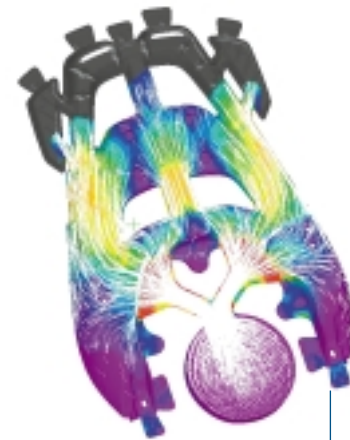
Velocity magnitude and new particle tracing display for an aluminum high pressure die casting application
