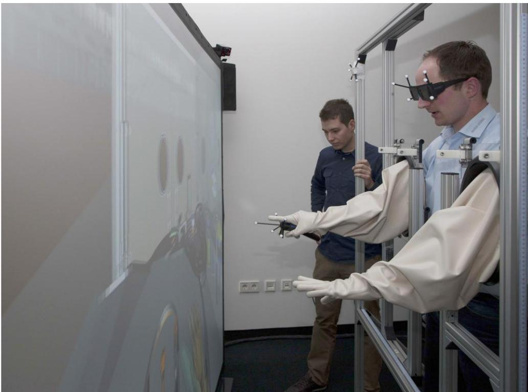
*Image: Virtual Mock-Up with IC.IDO Virtual Reality solution to evaluate reachability and visibility at Bausch & Stroebel*
