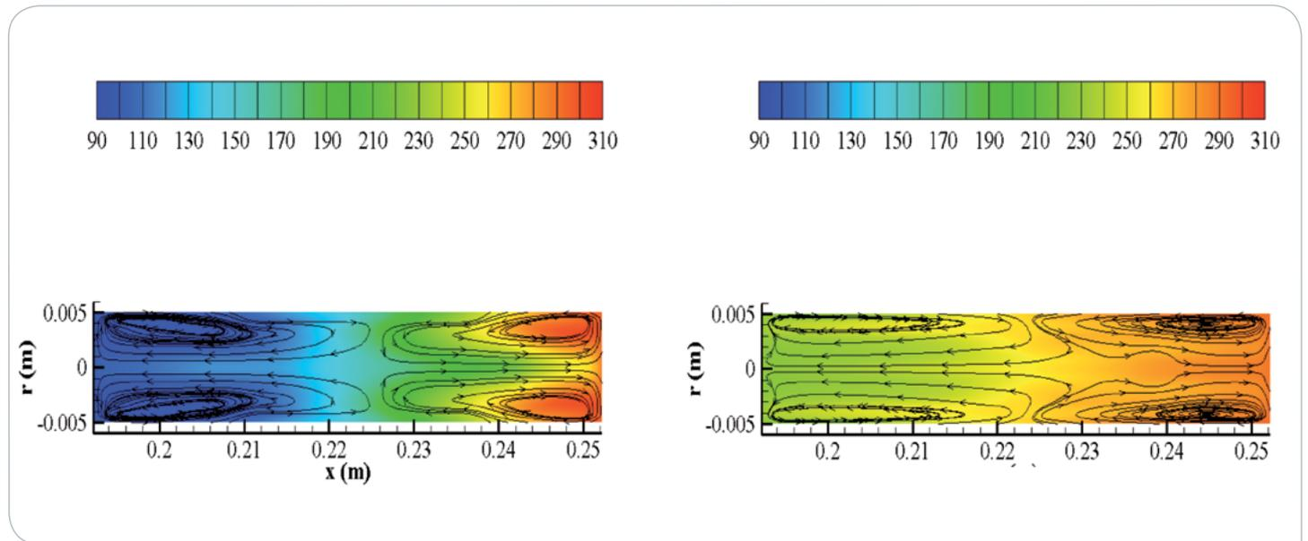
Figure 3: Flow and Temperature Profiles in "Pulse Tube" section of the cryocooler before (left) and after (right) the design changes.
