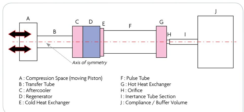
Figure 2: Model geometry of the Orifice Pulse Tube Refrigerator (OPTR).
