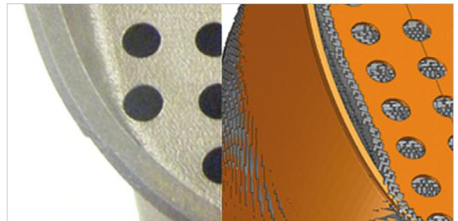
Simulation in ESI Additive Manufacturing shows distortion of the anti-sloshing grid due to incorrect geometry design and build orientation
