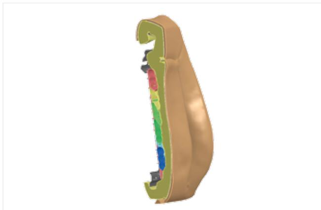
Fig.3: Inflation of the pneumatic bladder system
