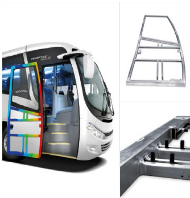
Fig. 1: Comil's Versatile vehicle and its door frame.
