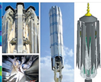
Fig. 4: Left to right: Folding and stowing of real umbrella, Stowing Simulation.
