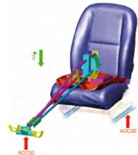
Experimental set-up and Finite Element model with Virtual Seat Solution.
