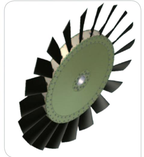
CAD model of the rotor with its 20 blades
