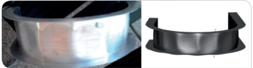
Fig. 1: Reality vs. simulation with PAM-STAMP 2G on an extreme bending case. The simulation properly forecasted defects.
