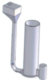
Fig. 1 - Thin walled Steel prototype casting
