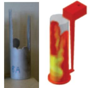
Fig. 2 - Trial run of partially filled prototype casting vs. Simulation results showing favorable correlation. (Using a different set of parameters than Fig. 2)
