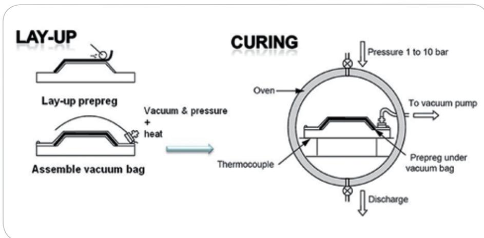
Composite mold manufacturing process
