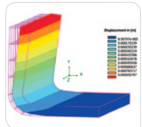
Predicted spring-in due to residual stresses release at the end of the manufacturing process
